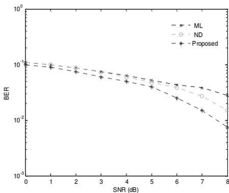
Figure 9. Comparison of BER versus SNR (dB) curves for a synchronous BPSK/DS CDMA system in a Gaussian channel for a small value of  $K$ .
